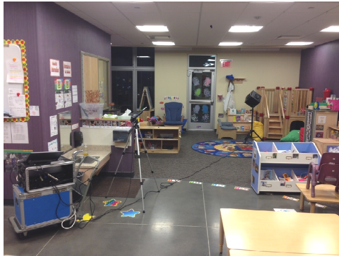
Figure 3-2: Typical Room Impulse Response Measurement Setup
